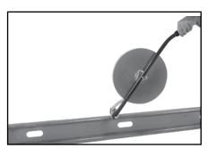
Install Gasket Tape on metal or wood studs or floor joists.
