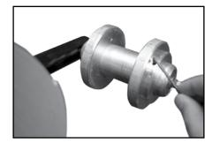
Adjust with 8 " Allen wrench to fit Gasket Tape.
